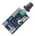
• **Stereo Output**: Dual-channel output delivers 2 × 30W of clean, high-quality audio.
